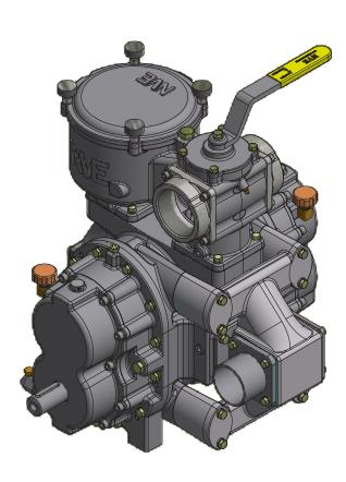
\*The maximum allowable operating vacuum will vary depending on R.P.M., ambient temperature, altitude and time running. The basic principle to keep in mind is - faster R.P.M., higher air temperature and longer run time all equal more heat in blower. When installing a NVE B500 blower we recommend a normal R.P.M. of 2400. Other speeds are ok as long as exhaust gas temperatures read on the supplied thermometer do not exceed 380 degrees F.
