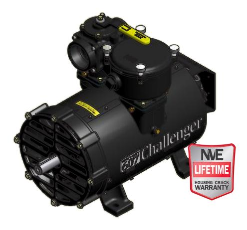
\*The maximum allowable operating vacuum will vary depending on R.P.M., ambient temperature, altitude and time running. The basic principle to keep in mind is - faster R.P.M., higher air temperature and longer run time all equal more heat in pump. When installing an NVE 607 pump we recommend a normal R.P.M. of 1250. Other speeds are ok as long as exhaust gas temperatures read on the supplied thermometer do not exceed 380 degrees F.
