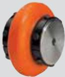
It is important to have a "break away" coupler insert to avoid catastrophic damage in the event the vacuum pump seizes. Improper alignment of the coupler will cause vibration and premature wear. Too much thrust pressure on the pump coupler can cause rotor to endplate contact on the pump non-drive end.
