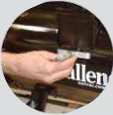
The Challenger pump is equipped with a vane wear inspection port. Vane wear is dependent upon many factors, though under normal conditions they should last approximately 2,000 hours. A vane is worn to the point of replacement when it is 1/4" below the rotor surface.
